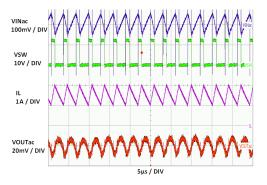
Figure 2. 1.5A-Load Steady State Operation
