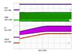
Figure 5. 1.5A-Resistive-Load Startup Via Enable Operation
