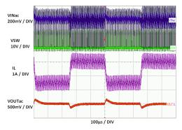
Figure 4. Transient Load Response
