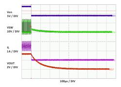
Figure 6. 1.5A-Resistive-Load Shutdown Via Enable Operation
