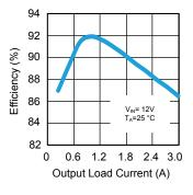
Figure 8. Efficiency as a Function of Load
