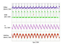
Figure 1. No-Load Steady State Operation
