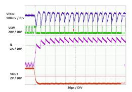
Figure 7. Short Circuit Entry Operation
