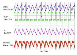
Figure 3. 3A-Load Steady State Operation
