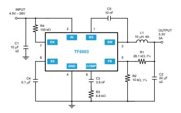
Figure 9. Typical Application Circuit
